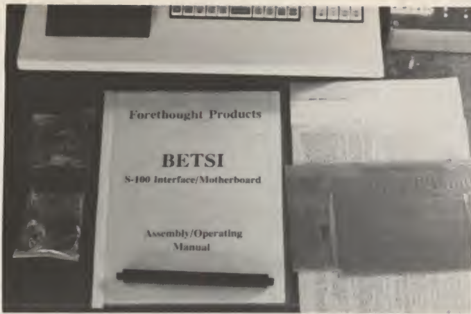
The Betsi kit. Here's all it takes to put your PET on the S-100 bus.
